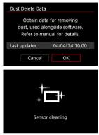
After the automatic self-cleaning of the image sensor is performed, a message will appear. Although there will be a mechanical sound of the shutter during the cleaning, no picture is taken.
