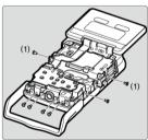
• There is no need to remove the small screws next to screw (1).
