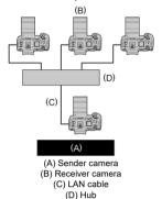
Use a highly shielded Category 5e or higher STP (Shielded Twisted Pair) Gigabit Ethernet cable.
