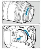
Remove the rear lens cap and the body cap by turning them as shown by the arrows.
