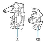
The cable protector consists of the protector (1) and a clamp (2).
