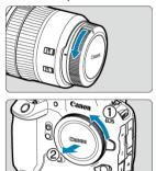
Remove the rear lens cap and the body cap by turning them as shown by the arrows.
