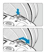
Press a button such as < MODE >, < DRIVE •AF >, <  $\bullet$  •  $\bullet$  >, or < M-F $\eta$  >, then turn the <  $\circ$  > dial.
